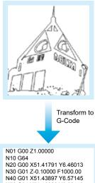
N20 G00 X51.41791 Y6.46013 N30 G01 Z-0.10000 F1000.00 N40 G01 X51.43887 Y6.57145 N50 G01 X51.46328 Y6.60449 N60 G01 X54.19628 Y9.64749 N70 G01 X54.54002 Y10.03007 N80 G01 X54.61772 Y10.20689 N90 G01 X54.69736 Y10.58087 N100 G01 X55.02240 Y12.08614 N110 G01 X55.22240 Y12.08614 N120 G01 X55.52968 Y12.78773
