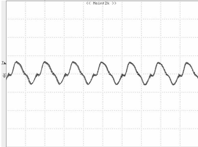
**Figure 14:** Output voltage ripple at nominal input voltage and rated load current ( $I_o=20A$ ) (20 mV/div, 2 us/div)
