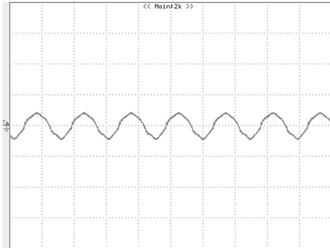
**Figure 11:** Input Terminal Ripple Current,  $i_c$ , at full rated output current and nominal input voltage with  $12\mu\text{H}$  source impedance and  $33\mu\text{F}$  electrolytic capacitor (500 mA/div, 2 us/div)
