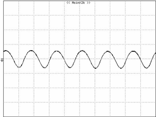
**Figure 9:** Input Terminal Ripple Current,  $i_c$ , at full rated output current and nominal input voltage ( $V_{in}=48v$ ) with 12 $\mu$ H source impedance and 33 $\mu$ F electrolytic capacitor (200 mA/div, 1 $\mu$ s/div)
