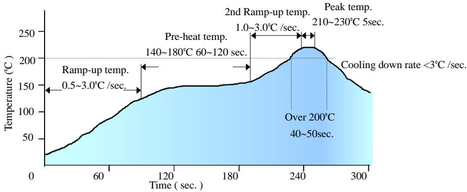
*Note: The temperature refers to the pin of V36SE, measured on the pin +Vout joint.*
