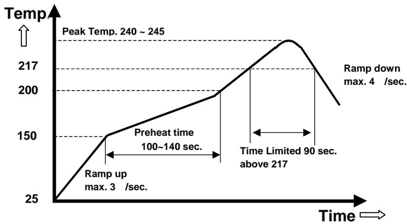
*Note: The temperature refers to the pin of V36SE, measured on the pin +Vout joint.*
