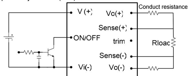
Figure 15: Effective circuit configuration for remote sense operation
