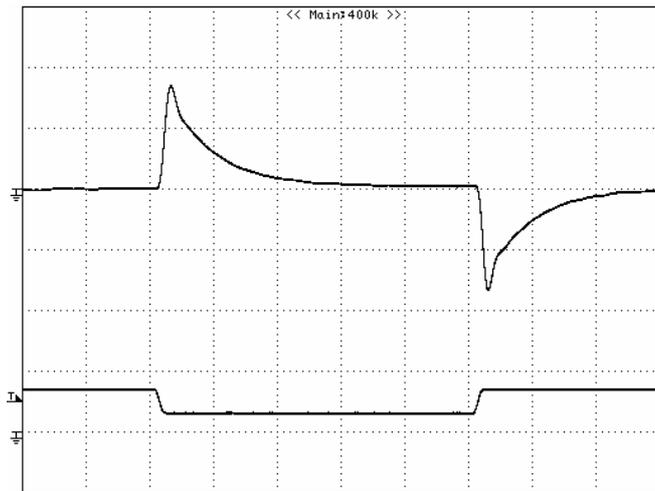
**Figure 6:** Output voltage response to step-change in load current (50%-25%-50% of  $I_{o, max}$ ;  $di/dt = 0.1A/\mu s$ ;  $V_{in}$  is 24v). Load cap: 10 $\mu F$  tantalum capacitor and 1 $\mu F$  ceramic capacitor. Top Trace:  $V_{out}$  (50mV/div, 200 $\mu s$ /div), Bottom Trace:  $I_{out}$  (5A/div). Scope measurement should be made using a BNC cable (length shorter than 20 inches). Position the load between 51 mm to 76 mm (2 inches to 3 inches) from the module
