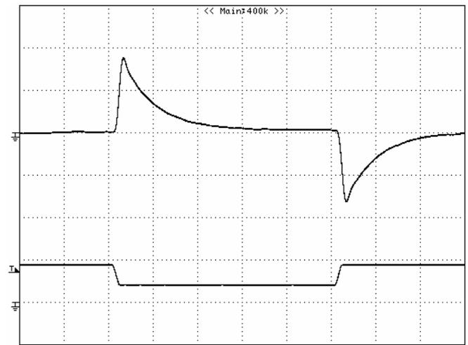
**Figure 7:** Output voltage response to step-change in load current (50%-25%-50% of  $I_{o, max}$ ;  $di/dt = 0.1A/\mu s$ ;  $V_{in}$  is 48v). Load cap: 10 $\mu F$  tantalum capacitor and 1 $\mu F$  ceramic capacitor. Top Trace:  $V_{out}$  (50mV/div, 200 $\mu s$ /div), Bottom Trace:  $I_{out}$  (5A/div). Scope measurement should be made using a BNC cable (length shorter than 20 inches). Position the load between 51 mm to 76 mm (2 inches to 3 inches) from the module
