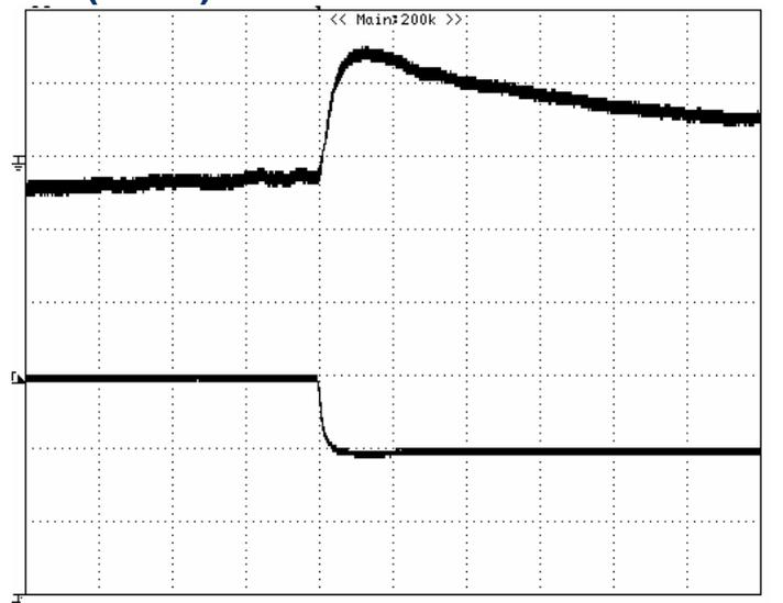
**Figure 8:** Output voltage response to step-change in load current (75%-50% of  $I_{o, max}$ ;  $di/dt = 0.1A/\mu s$ ). Load cap: 10 $\mu F$  tantalum capacitor and 1 $\mu F$  ceramic capacitor. Top Trace:  $V_{out}$  (100mV/div, 100 $\mu s$ /div), Bottom Trace:  $I_{out}$  (0.5A/div). Scope measurement should be made using a BNC cable (length shorter than 20 inches). Position the load between 51 mm to 76 mm (2 inches to 3 inches) from the module.
