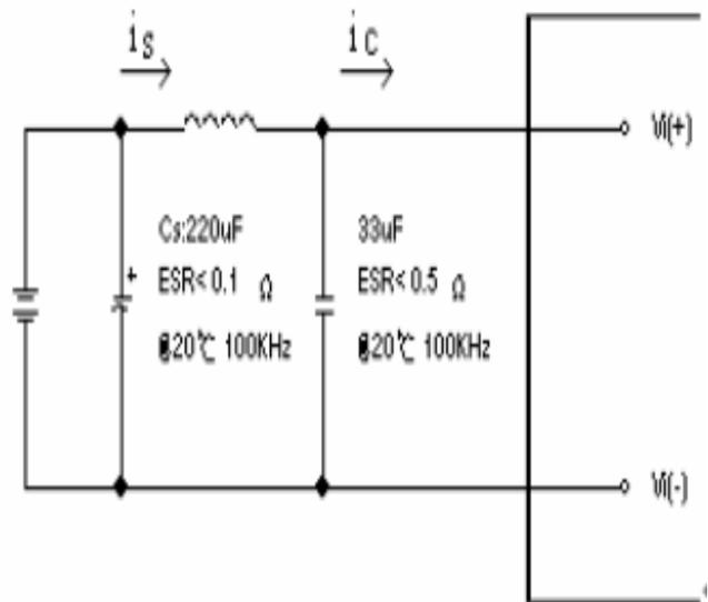
**Figure 10:** Test set-up diagram showing measurement points for Input Terminal Ripple Current and Input Reflected Ripple Current. Note: Measured input reflected-ripple current with a simulated source Inductance ( $L_{TEST}$ ) of  $12\mu H$ . Capacitor  $C_s$  offset possible battery impedance. Measure current as shown below.
