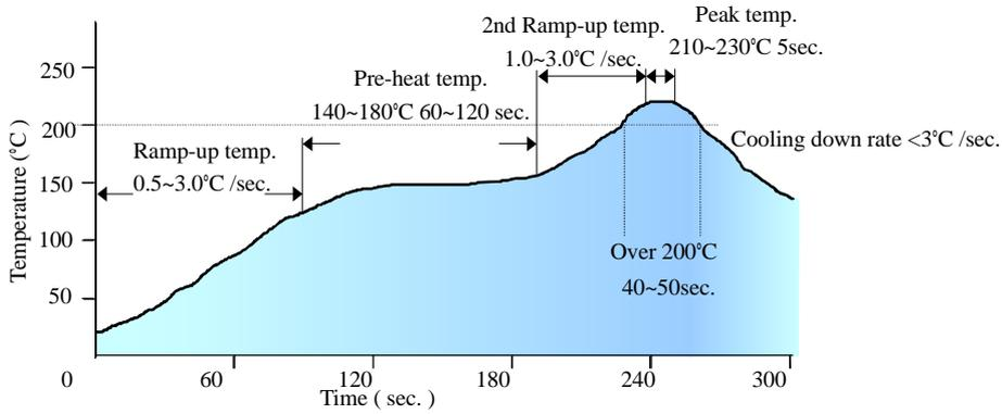
*Note: The temperature refers to the pin of S36SE, measured on the pin +Vout joint.*
