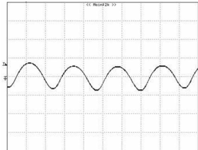
**Figure 11:** Input Terminal Ripple Current,  $i_c$ , at full rated output current and nominal input voltage with  $12\mu H$  source impedance and  $33\mu F$  electrolytic capacitor (20mA/div, 1us/div)
