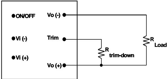
**Figure 17:** Circuit configuration for trim-down (decrease output voltage)
