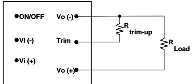
**Figure 18:** Circuit configuration for trim-up (increase output voltage)
