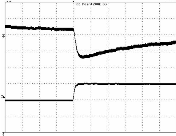
**Figure 9:** Output voltage response to step-change in load current (50%-75% of  $I_o$ , max;  $di/dt = 0.1A/\mu s$ ). Load cap:  $10\mu F$  tantalum capacitor and  $1\mu F$  ceramic capacitor. Top Trace:  $V_{out}$  (100mV/div, 100us/div), Bottom Trace:  $I_{out}$  (0.5A/div). Scope measurement should be made using a BNC cable (length shorter than 20 inches). Position the load between 51 mm to 76 mm (2 inches to 3 inches) from the module.
