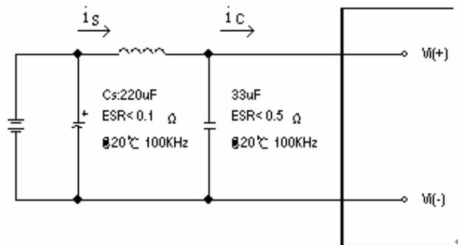
**Figure 10:** Test set-up diagram showing measurement points for Input Terminal Ripple Current and Input Reflected Ripple Current. Note: Measured input reflected-ripple current with a simulated source Inductance ( $L_{TEST}$ ) of  $12\mu H$ . Capacitor  $C_s$  offset possible battery impedance. Measure current as shown below.
