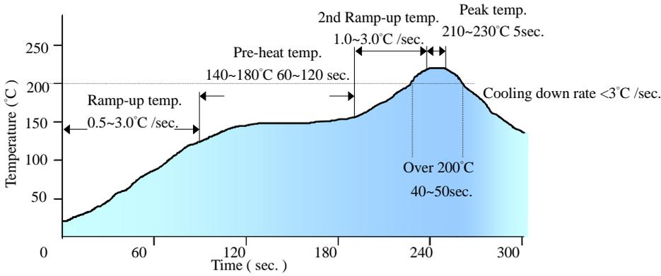
*Note: The temperature refers to the pin of S36SE, measured on the pin +Vout joint.*
