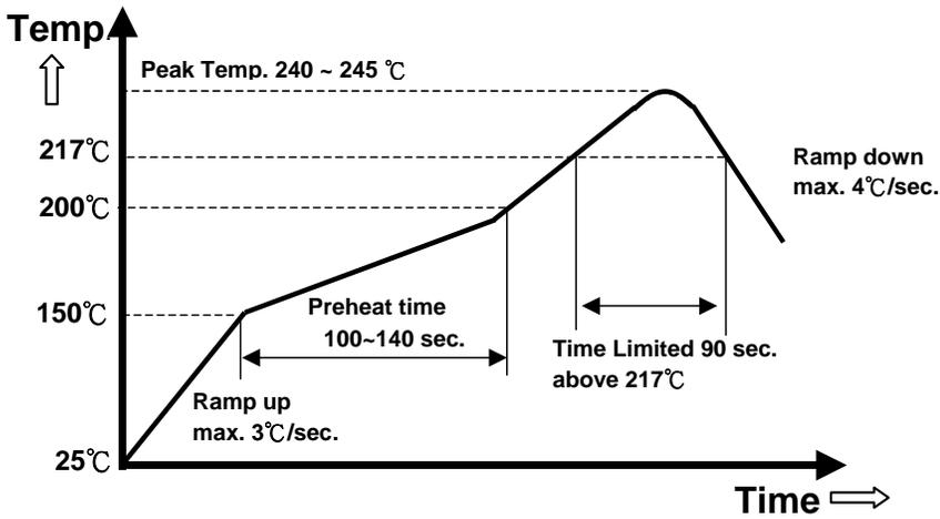
*Note: The temperature refers to the pin of S36SE, measured on the pin +Vout joint.*
