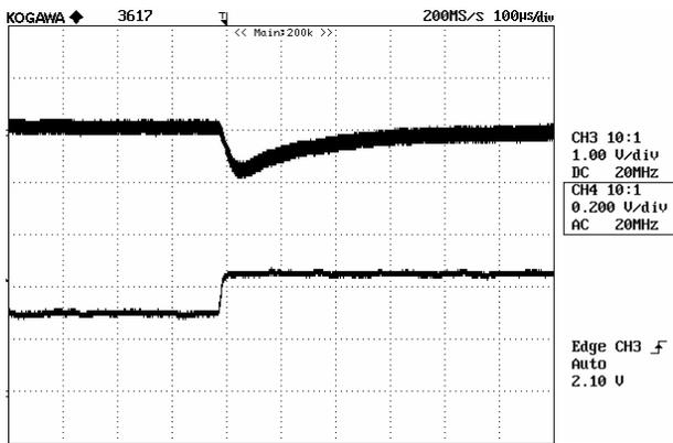
**Figure 9:** Output voltage response to step-change in load current (50%-75% of  $I_o$ , max;  $di/dt = 0.1A/\mu s$ ). Load cap:  $10\mu F$  tantalum capacitor and  $1\mu F$  ceramic capacitor. Top Trace:  $V_{out}$  (200mV/div, 100us/div), Bottom Trace:  $I_{out}$  (1A/div). Scope measurement should be made using a BNC cable (length shorter than 20 inches). Position the load between 51 mm to 76 mm (2 inches to 3 inches) from the module.
