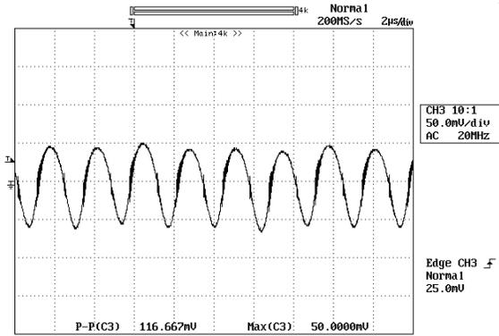
**Figure 11:** Input Terminal Ripple Current,  $i_c$ , at full rated output current and nominal input voltage with  $12\mu\text{H}$  source impedance and  $33\mu\text{F}$  electrolytic capacitor (50mA/div, 2us/div)
