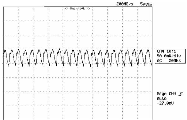
**Figure 14:** Output voltage ripple at nominal input voltage and rated load current ( $I_o=3\text{A}$ ) (50 mV/div, 5us/div). Load capacitance:  $1\mu\text{F}$  ceramic capacitor and  $10\mu\text{F}$  tantalum capacitor. Bandwidth: 20 MHz. Scope measurements should be made using a BNC cable (length shorter than 20 inches). Position the load between 51 mm to 76 mm (2 inches to 3 inches) from the module
