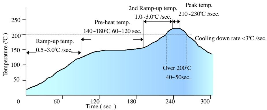
*Note: The temperature refers to the pin of E36SR, measured on the pin +Vout joint.*
