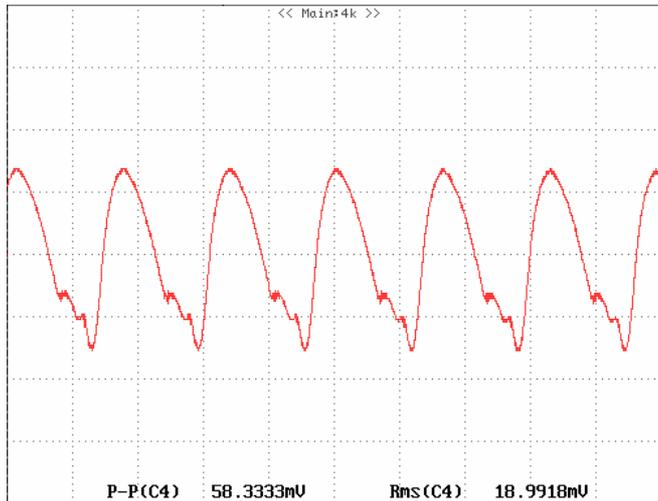
**Figure 14:** Output voltage ripple at  $48\text{V}_{\text{in}}$  and rated load current ( $I_o=20\text{A}$ ) ( $20\text{ mV/div}$ ,  $2\mu\text{s/div}$ )
