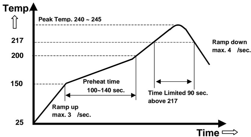
*Note: The temperature refers to the pin of E36SR, measured on the pin +Vout joint.*
