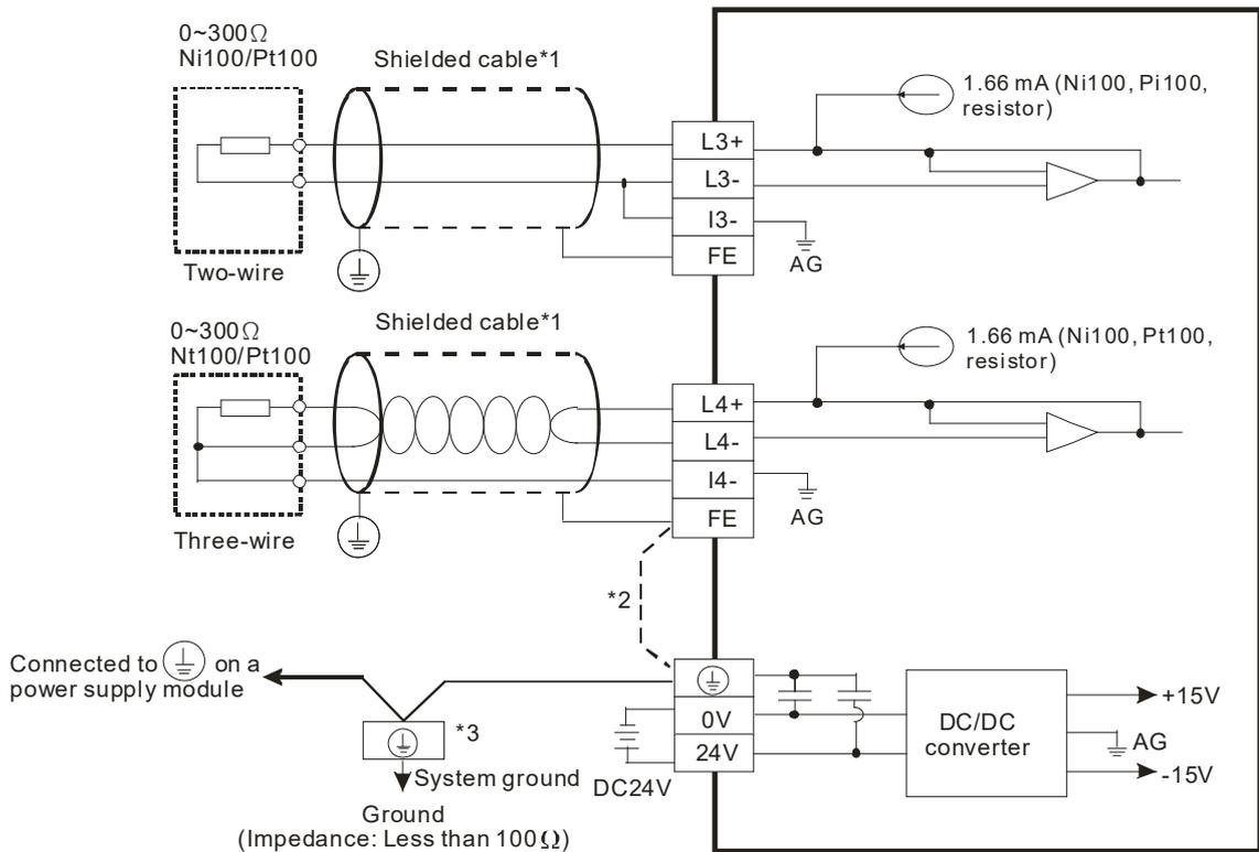
\*1: The cables connected to the input terminals should be cables or shielded twisted pair cables which can be connected to temperature sensors, and should be kept separate from other power cables and cables which may generate noise.
