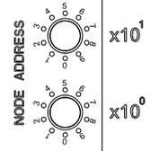
Example: If you need to set the node address of RTU-DNET to 26, simply switch the corresponding switch of  $x10^1$  to 2 and the corresponding switch of  $x10^0$  to 6.
