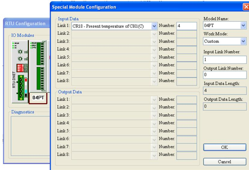
Explanation of special module setup parameters:
