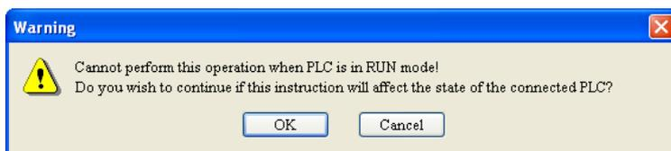
4. Click on “OK” to continue the download. Make sure DVP-SV is in RUN mode. Now, you can see the MS LED and NS LED on RTU-DNET and DVP-SV become green. And LED nixie tube of DVPDNET shows “01”.
