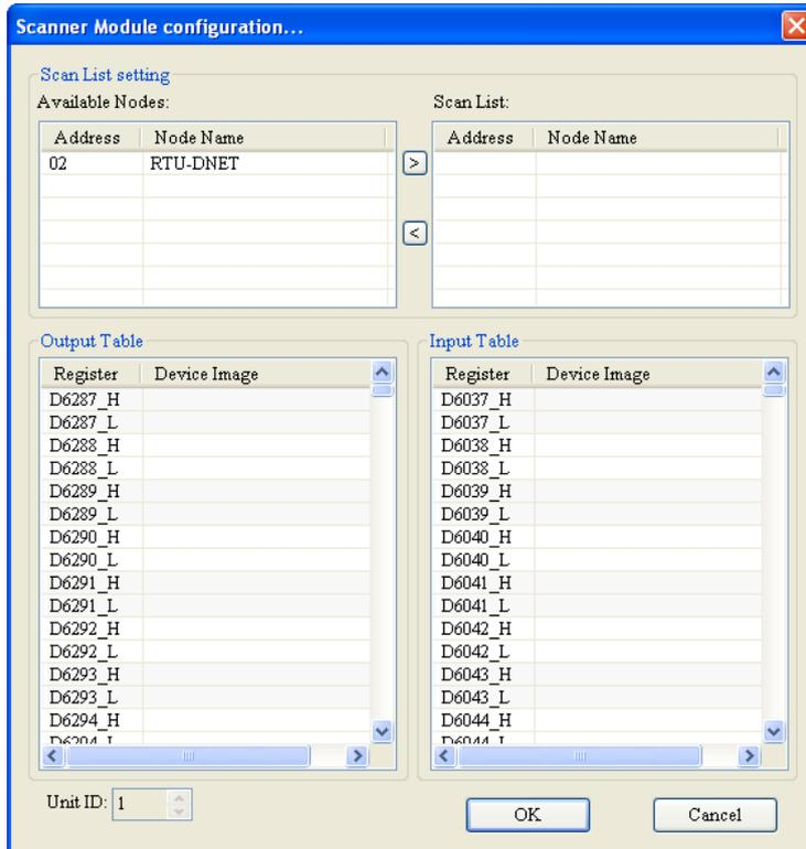
2. Move the slave devices on DeviceNet in the “Available Nodes” list on the left side to the “Scan List” on the right side. Select a node and click on
