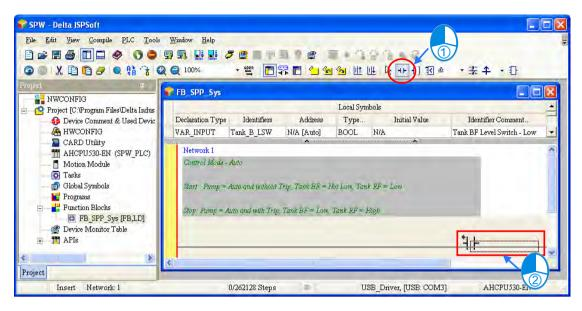
Click ???, and type "Pump\_Remote". When "Pump\_Remote" is typed, the drop-down list appears. Users can select the item directly, or type the words by themselves. After "Pump\_Remote" is typed, press the enter key.
