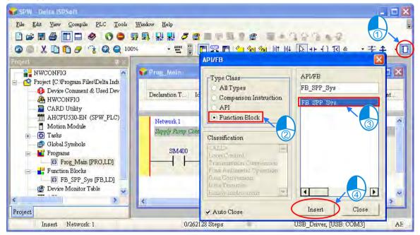
After the function block interface appears, type the identifiers as shown below.
