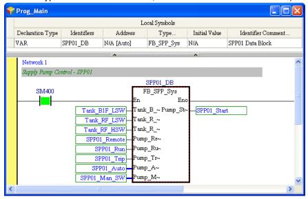
If users want to alter the value in the device, they can click the right mouse button. Tank\_B1F\_LSW is the device which is modified here. Please notice that the device corresponds to an actual I/O device. Setting the device to ON or OFF is meaningless because the actual I/O value covers the setting value immediately. To alter the value in the device, users need to force the device ON or OFF.
