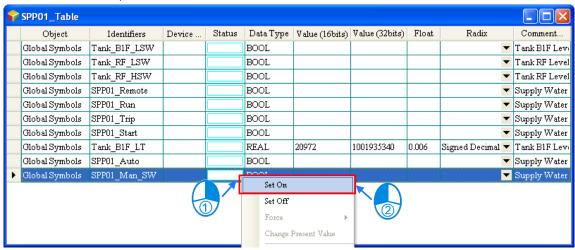
After the state of SPP01\_Man\_SW is altered, users can get the following device monitoring table.
