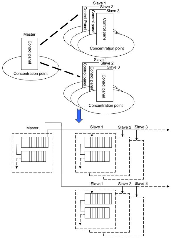
Note: The remote masters in DeviceNet are the network modules. They have to be installed with the CPU modules on the same backplane. A CPU module can support eight masters, and a master can be connected to sixty-three slaves. Besides, a slave can be connected to seven extension backplanes at most.
