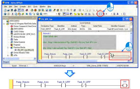
Click ???, and type "Pump\_Out". Users can double-click the coil marked "Pump\_Out", and the drop-down list appears. Select "Set".
