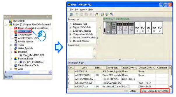
After users click , the **Transfer Items** window will appear. After the users click **OK**, the hardware configuration and the CPU parameters will be downloaded to the CPU module.
