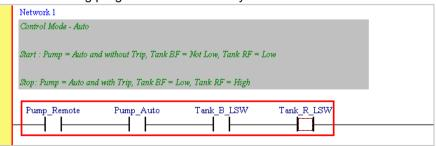
To meet the condition that there is water in the underground pool and no water in the water tower, the state of Tank\_R\_LSW should be OFF. Users can double-click the contact marked "Tank\_R\_LSW", and the drop-down list appears. Select "Normally Closed".
