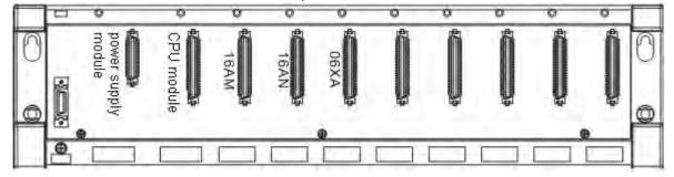
Connect the module to the connector on the backplane, make sure that the module is installed on the backplane properly, and tighen the the screw.
