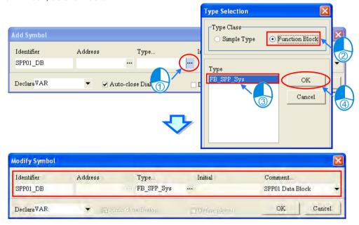
After the local symbol is created, the identifier can be given to the function block. (The data type should be the same with the name of the function block.)
