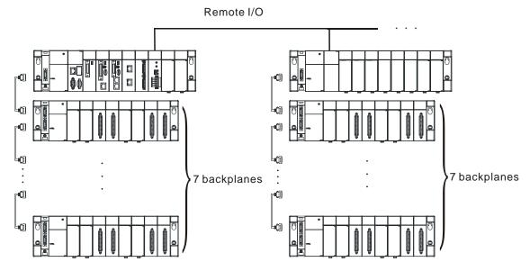
Note: Users are provided with the special cables to connect the extension backplanes. The length of a special cable can be up to 100 meters. They are also provided with the fiber cables which are used with the special adapters. The length of a fiber cable can be up to 2 kilometers.
