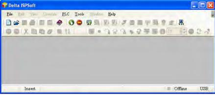
Step 2: Click to create a project. The example is related to the water supply, and therefore the project name is SPW. The PLC type is AHCPU530-EN, and the file path is the default path. Finally, click **OK**.
