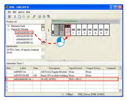
After the module is placed in the appropriate position, the system automatically distributes the addresses to the module. The default addresses are X0.0~X0.15. They exactly meet the need, and therefore they do not need to be modified. If they do not meet the need, users can click the column to modify the addresses.
