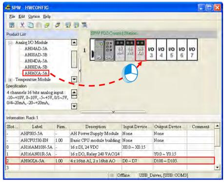
In addition to specifying the input device range and the output device range, users also have to specify the version of the firmware for the analog input/output module. Please select the version of the firmware according to the version of the firmware in the module.
