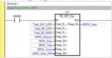
Users need to create a data block for the function block. The data block can be created as a global symbol or a local symbol, but it is created as a local symbol in the main program here. Notice that users need to select **Function Block** in the **Type Class** box, and select "FB\_SPP\_Sys" in the **Type** box. Please type "SPP01\_DB" in the **Identifier** box, and type "SPP01 Data Block" in the **Comment...** box, as show below.
