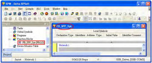
Users need to create the local symbols. In order to make the use of the function block more convenient, the system automatically distributes the addresses to the module, and users are not
