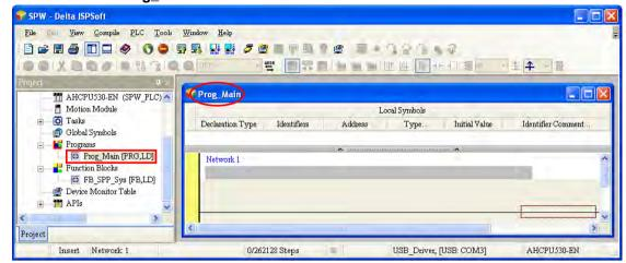
The difference between the function block and the main program is that the function block has to be called before it is executed while the main program is executed directly. The creation of the local symbols for the main program is omitted in this example. Please write the following program by means of the skills learned previously.
