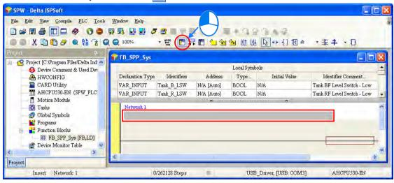
Type the following description as the comment on network 1. If users want to start a new line of text at a specific point, they can press Alt+Enter on the keyboard.
