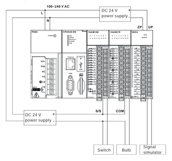
The wiring of the modules is described in detail below. (Please refer to AH500 Hardware Manual for more information.)
