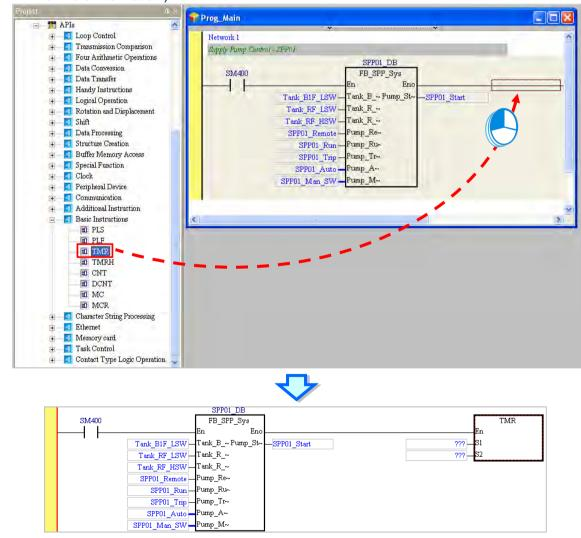
If users need to create the second system, they only need to call "FB\_SPP\_Sys" again, and type the identifier. Please notice that the same data block can not be used in the two systems unless user
