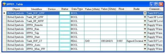
If users want to alter the value in the device, they can click the right mouse button. The state of SPP01\_Man\_SW is altered here. Owing to the fact that the device does not correspond to an actual I/O device, users can set the device to ON or OFF.
