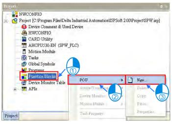
Type "FB\_SPP\_Sys" in the **POU Name** box, and then type "Supply Water Pump Control Function" in the **POU Comment** box. Finally, click **OK**.
