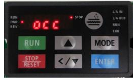
Here are two images of KPVJ-LE02 displaying unusual signals. On the left, it shows the number of the unusual signals. On the right, it shows the name of the unusual signal. The KPVJ-LE02 switches automatically back and forth between these two ways of displaying the unusual signal.
