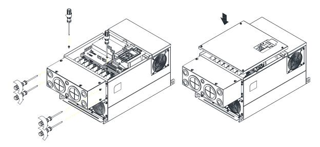
3. Fasten the 4 screws shown in the following figure. Screw torque: 12–15 kg-cm / (10.4–13 lb-in.) / (1.2–1.5 Nm)
