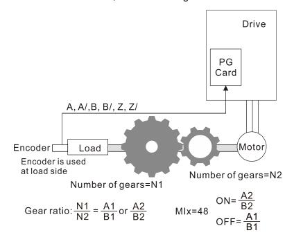
A1 = Mechanical Gear A1 at Load Side (Pr.10-04)
