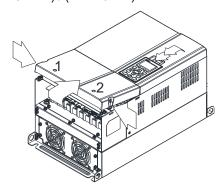
(Figure 2) Loosen screw 3; press the tab on the right and the left to remove the cover. Screw 3 Torque: 6–8 kg-cm / (5.2–6.9 lb-in.) / (0.6–0.8 Nm)
