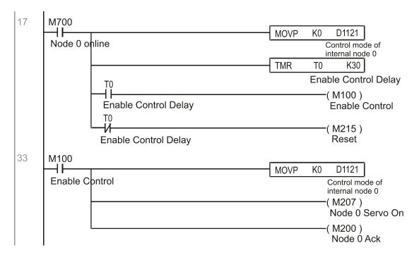
It is required slave station 1 maintains forward rotation at 30.00 Hz for 1 sec., and maintains reverse rotation at 60.00 Hz for 1 sec., and repeat this cycle continuously.
