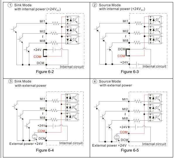
☑ When the photo-coupler uses the internal power supply, the switch connection for Sink and Source modes shows as Figure 6-2 and Figure 6-3:
