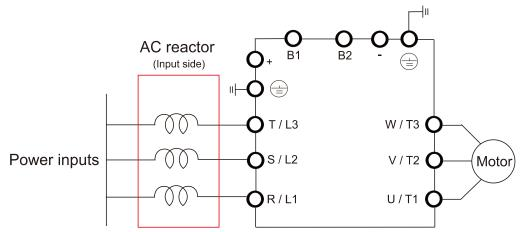
Figure 7-5 Wiring an AC input reactor
