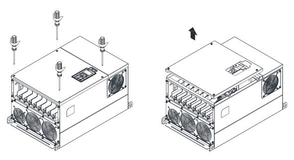
2. Fasten the 6 screws shown in the following figure and place the cover back to the original position. Screw torque: 24–26 kg-cm / (20.8–22.6 lb-in.) / (2.4–2.5 Nm)
