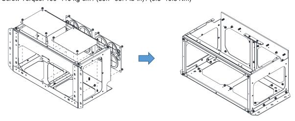
3. Remove the parts and screws as below figure shown.
