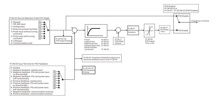
Master Frequency Command Source (AUTO) / Source Selection of the PID Target
