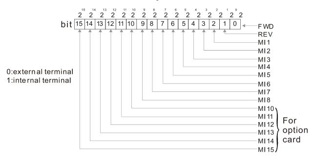
Setting method: convert the binary 12bit number to hexadecimal number for input. Example: if the MI1, MI3, MI4 are virtual terminals, Pr.02-74 = 34h.
