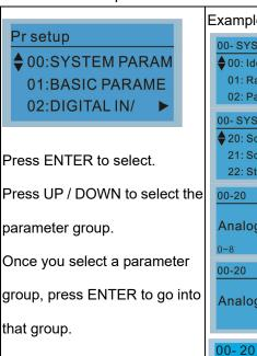
Example: Setup source for the master frequency command.
