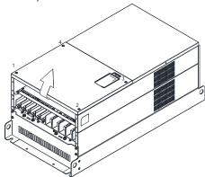
Loosen screw 1, 2, 3 and remove the protective ring (as shown in figure 3) Screw torque: 14–16 kg-cm / (12.2–13.9 lb-in.) / (1.4–1.6 Nm)
