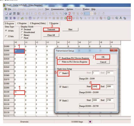
(3) Another method can be used to set D1091: Determine which of slave stations 0 to 7 will not be needed, and set the corresponding bits to 0. For instance, if it is not necessary to control slave stations 2, 6 and 7, merely set D1091 = 003B, and the setting method is the same as described above: Use WPL to initiate **communications** > **use register edit (T C D)** function to perform settings.
