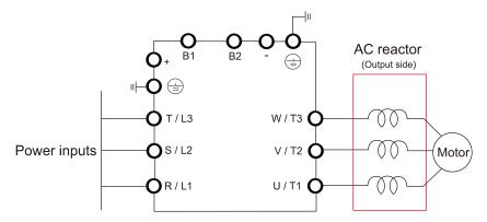
Figure 7-10 Wiring an AC output reactor
