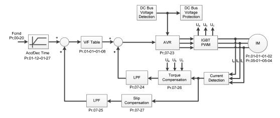
When Pr.00-10 = 0, and you set Pr.00-11 to 2, the space vector control diagram is as follows: IM Sensorless Vector Control (IMSVC):
