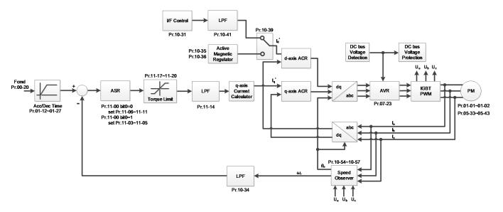
When Pr.00-10 = 0, and you set Pr.00-11 to 7, IPM FOC sensorless control diagram is as follows:
