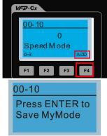
2. The parameter (Pr) displays in My mode if it is properly saved. To correct or to delete this parameter, press F4 for DEL.
