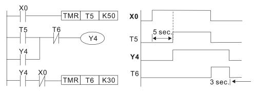
Example 12: Extended timing circuit
