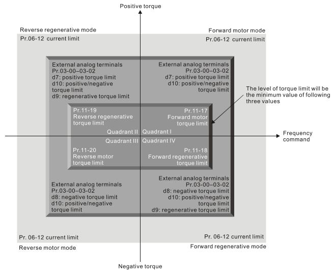
All control modes are based on 100% motor rated current except for these four modes: IM: VF, SVC / PM: PMSVC modes.
