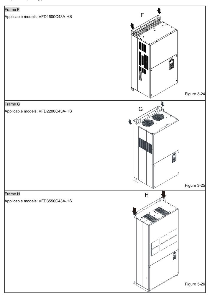
Ensure the lifting hook properly goes through the lifting hole, as shown in the following diagram.
