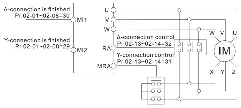
Y- $\Delta$  connection switch: can be used for wide range motor
