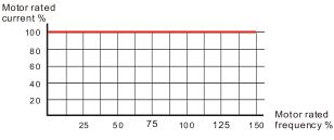
Motor cooling curve with shaft-fixed fan
