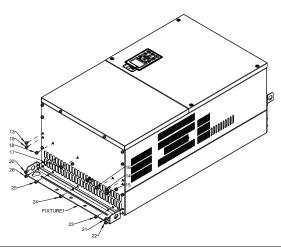
4. Install Fixture 1 by fasten screw 13–26 Screw torque: 24–26 kg-cm / (20.8–22.6 lb-in.) / (2.4–2.5 Nm)
