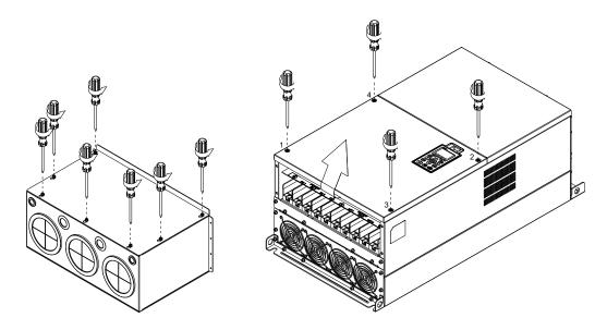
3. Remove the top cover and loosen the screws.
