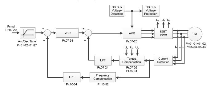
When Pr.00-10 = 0, and you set Pr.00-11 to 3, the IM FOCPG control diagram is as follows:
