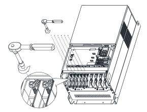
4. Install the 3pcs copper assy., as shown in the following figure 1. Fasten the upper M8 nuts (1–6) with a sleeve wrench (12 mm of the sleeve), as shown in the figure 2 and figure 3 below.
