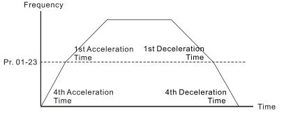
1st/4th Acceleration/Deceleration Frequency Switching
