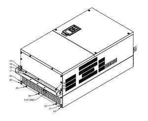
5. Place 4 of the M12 screws through Fixture 1&2 and plate then fasten the screws. Screw torque: 300–400 kg-cm / (260–347 lb-in.) / (29.4–39.2 Nm)
