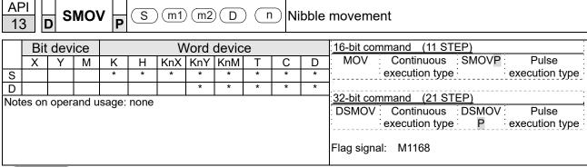
**S**: Data source. **m**<sub>1</sub>: The data source transfers starting bit number.
