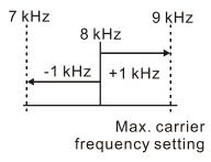
When Pr.00-17 = 5, 6, or 7 kHz, the maximum setting for Pr.00-34 is 4.0 kHz (±2 kHz). The carrier frequency fluctuation range is according to the diagram below.
