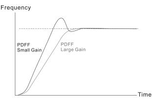
11-14 ASR Output Low Pass Filter Time Default: 0.008 Settings 0.000-0.350 sec. Sets the ASR command filter time. **11-15** Notch Filter Depth Default: 0 Settings 0-100 dB Notch Filter Frequency Default: 0.00 Settings 0.0-6000.0 Hz 11-47 Notch Filter Bandwidth Default: 0 Settings 0-1000 Hz
