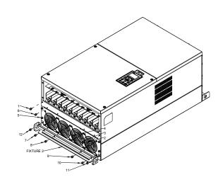
Loosen 12 screws and remove Fixture 2.
