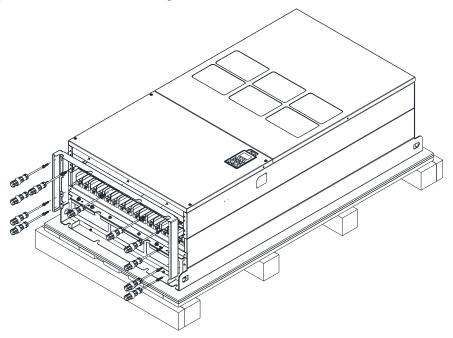
4. Fasten the M6 screws to locations shown in below figure.
