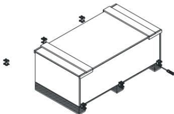
Step 1: Unscrew all the cover screws (24 screws).
