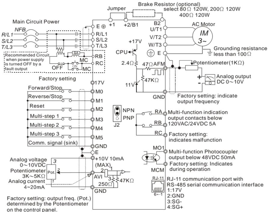
○ Main circuit (power) terminals    ⊙ Control circuit terminals    ◻ Shielded leads
