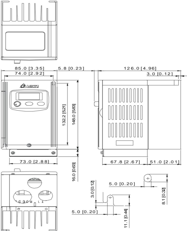
Frame S1: VFD002S21E, VFD004S21E, VFD007S21E, VFD015S23D
