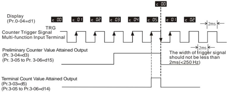
**3-05** Multi-function Output Terminal 1 (Photocoupler output)
