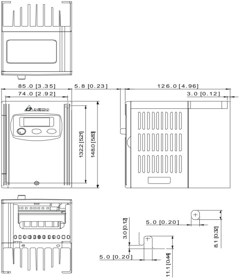
Frame S1: VFD004S43B, VFD007S43B
