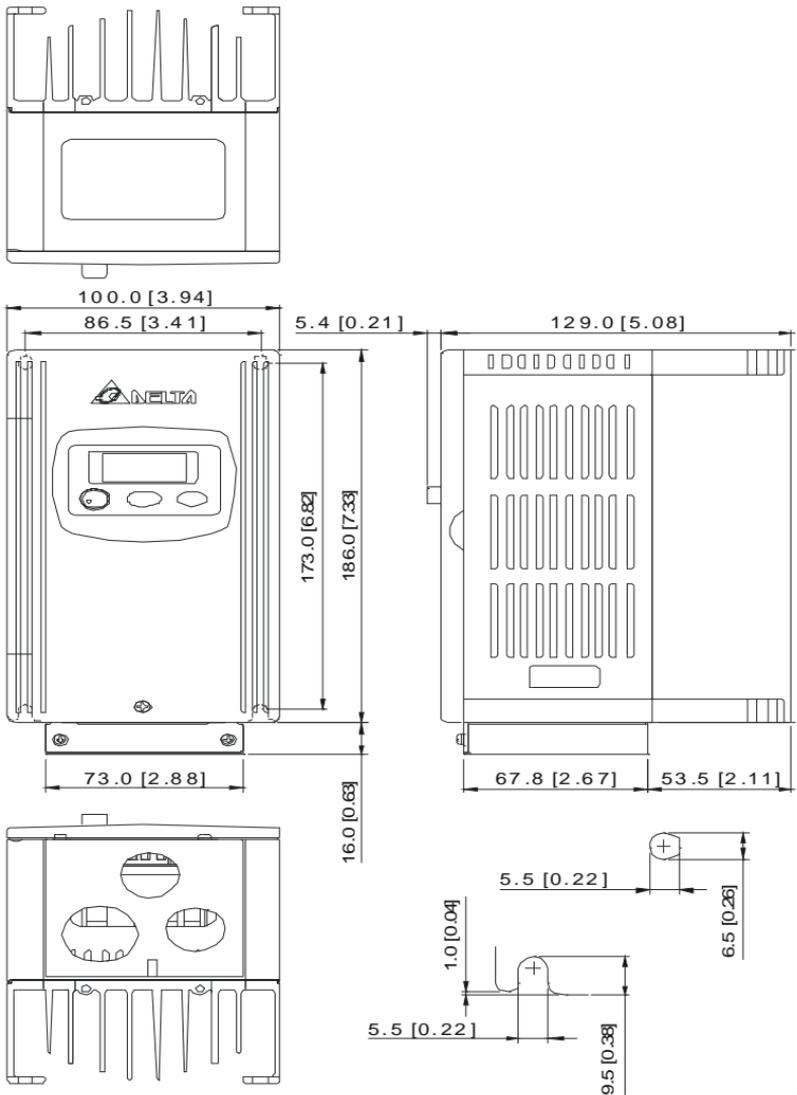
Frame S2: VFD015S21D, VFD015S21E, VFD015S43D, VFD015S43E, VFD022S21D,
