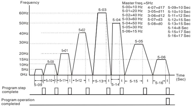
**Example 4 (Pr. 5-07 =d4) Continuously execute PLC cycles step by step:**
