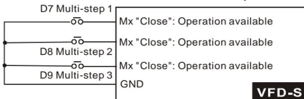
These three inputs select the multi-step speeds defined by Pr.5-00 to Pr.5-06 as shown in the following diagram. Pr.5-07 to Pr.5-16 can also control output speed by programming the AC drive's internal PLC function.
