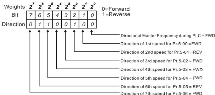
The setting value =  $\text{bit7} \times 2^7 + \text{bit6} \times 2^6 + \text{bit5} \times 2^5 + \text{bit4} \times 2^4 + \text{bit3} \times 2^3 + \text{bit2} \times 2^2 + \text{bit1} \times 2^1 + \text{bit0} \times 2^0$
