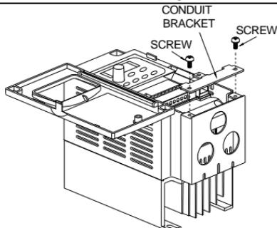
Install Conduit Bracket cover and tighten screws.
