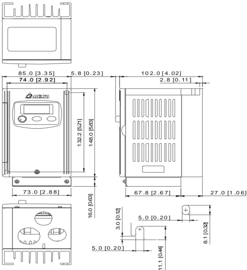
Frame S1: VFD007S21A, VFD007S23A
