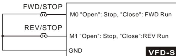
**d2 Two wire operation:** Restrict to Pr. 4-04 and external terminals M0, M1.
