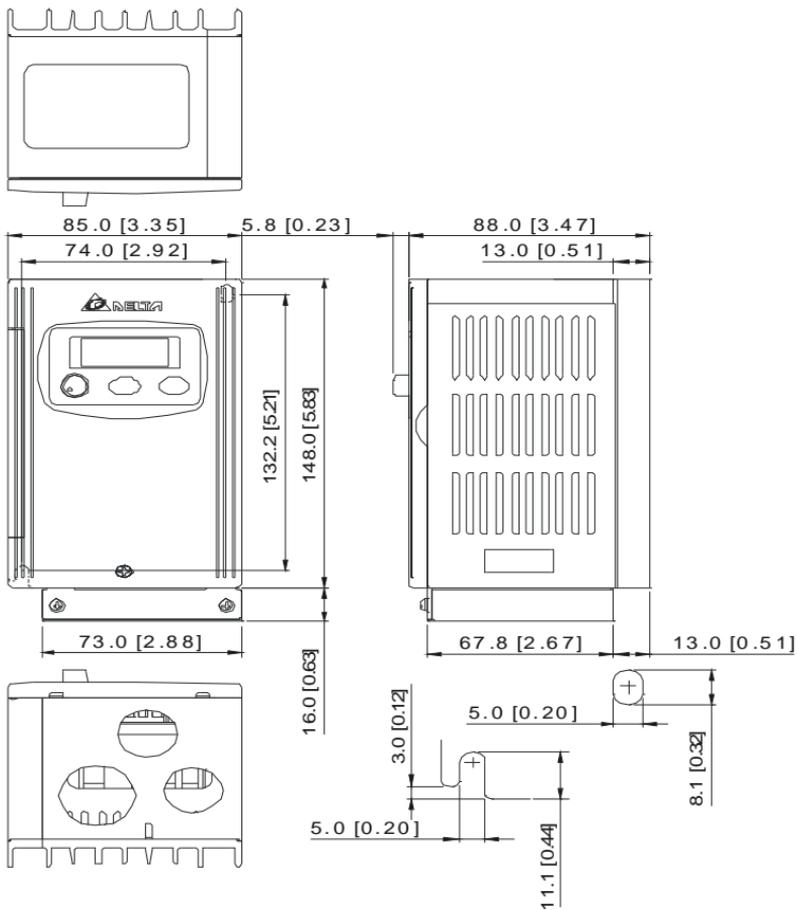
Frame S1: VFD004S11A, VFD004S21A, VFD004S23A
