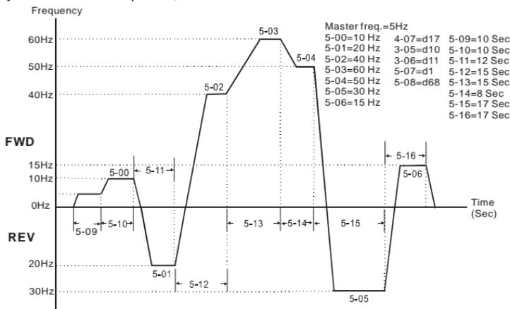
\* The calculation of time for Pr.5-11, Pr.5-12, Pr.5-15 and Pr.5-16 should be carefully planned.
