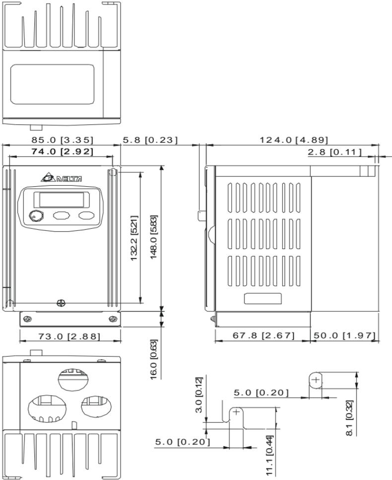
Frame S1: VFD004S43A, VFD004S43E, VFD007S43A, VFD007S43E
