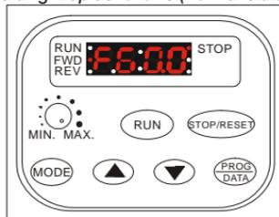
When power is ON, LEDs "STOP" and "FWD" should light up. The display will show "F60.0".
