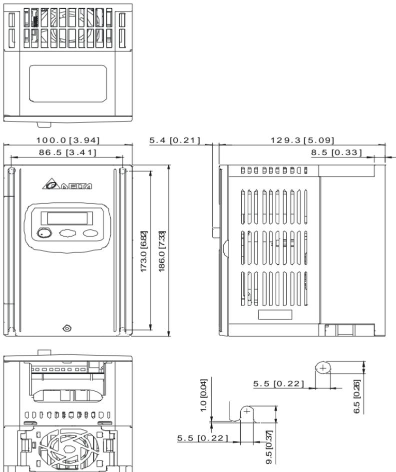
Frame S2: VFD015S21U, VFD015S43U, VFD022S21U, VFD022S43U
