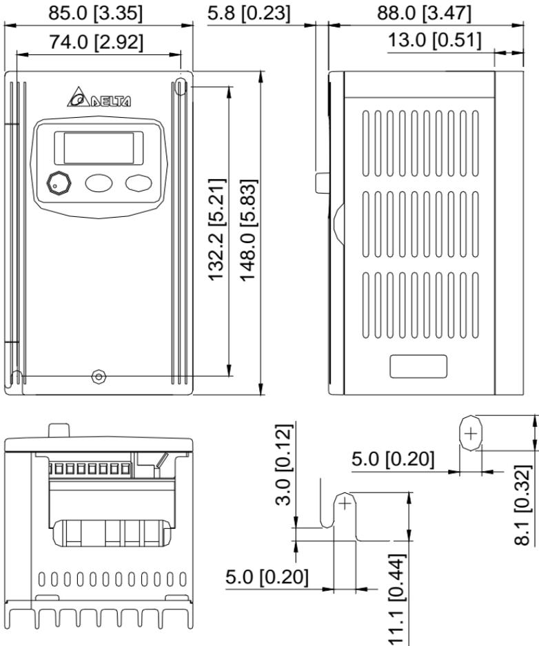
Frame S1: VFD002S11B, VFD002S21B
