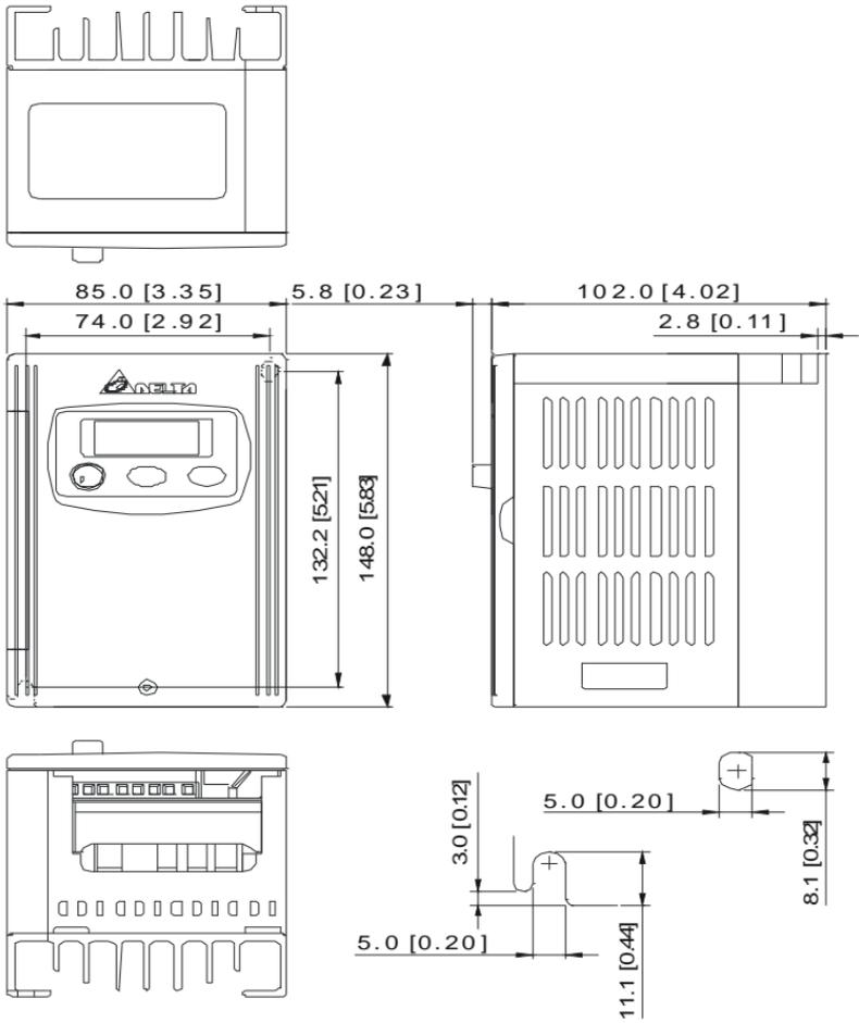
Frame S1: VFD004S11B, VFD004S21B
