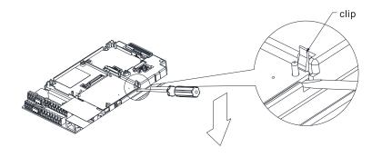
As shown in the figure on the left. Twist to open the clip. Insert a slot type screwdriver into the hollow to prize the PCB off the clip.
