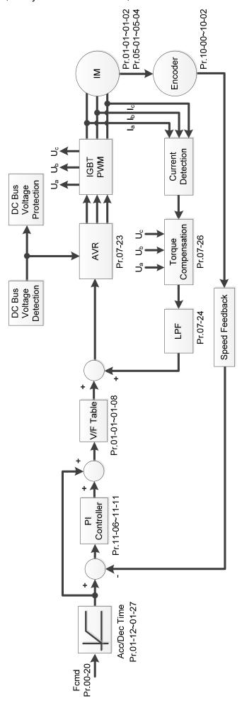
When Pr.00-10 = 0, and you set Pr.00-11 to 2, the space vector control diagram is as follows: IM Space Vector Control (IMSVC):
