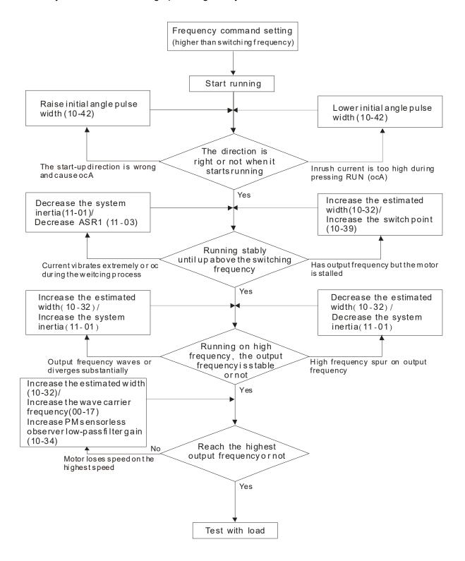
IPM sensorless control diagram
