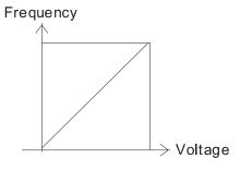
Fcmd=[(ay $\pm$ bias)\*gain]\*  $\frac{\text{Fmax}(01-00)}{10\text{V or }16\text{mA or }20\text{mA}}$
