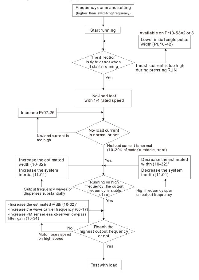
Flow chart of adjustment when starting up WITH load
