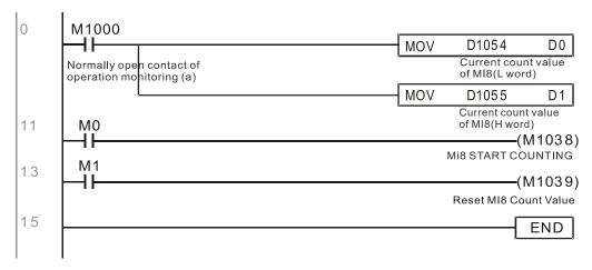
When the PLC program defines MI8 for use as a high-speed counter, and also for use in PLC procedures, it must be written to M1038 or M1039, and the original MI8 functions will be disabled.
