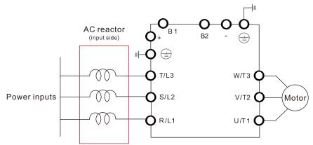
Figure 7-6 Wiring of AC input reactor
