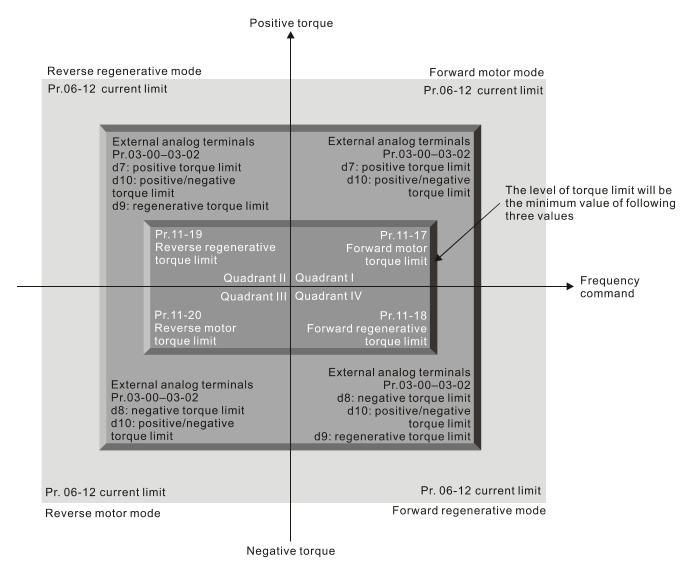
In IM: VF, VFDPG, SVC / PM, PMSVC modes, their 100% base values are the drive's rated current, but for other control modes, 100% base values are the motor's rated current.
