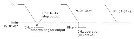
In FOCPG mode, when Pr.01-34 is set to 2, the AC motor drive operates according to this setting.
