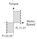
Forward Speed Limit (Torque Mode)
