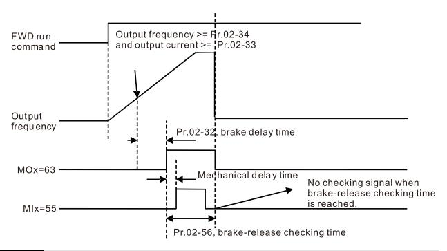
Multi-Function Output Terminal (Function 42): Brake Current Check Point
