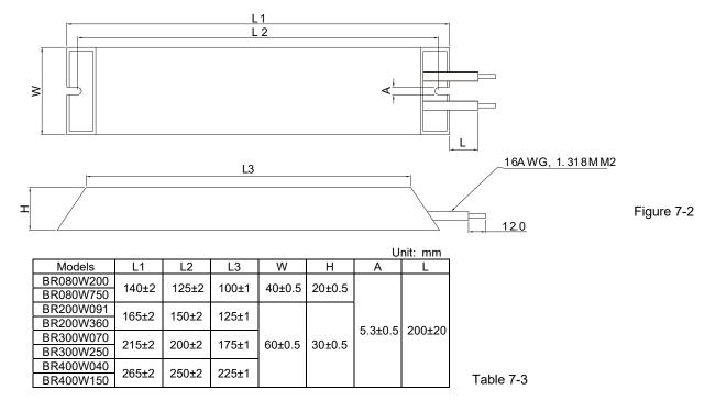
2. Select the resistance value, power and brake usage (ED %) according to Delta rules.
