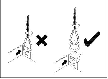
Pay attention to the angle between the lifting hole and the lifting hook, see the figure below. Applicable to VFD450CT43F00B; VFD550CT43F00B; VFD450CT43F00A3 VFD550CT43F00A4; VFD750CT43F00A6; VFD900CT43F00A8
