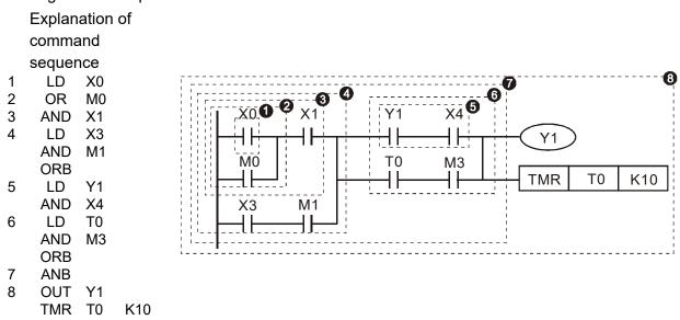
Explanation of basic structure of ladder diagrams
