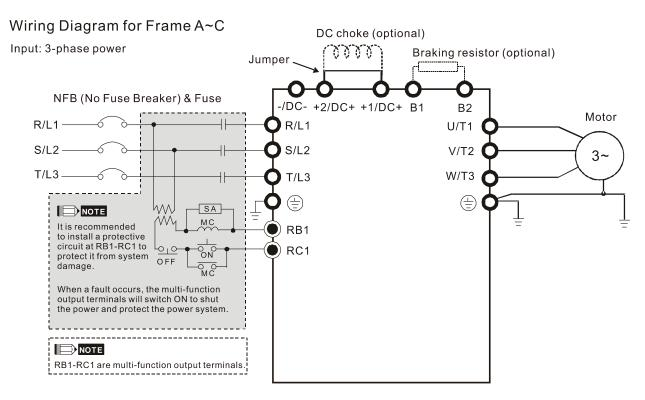
Figure 7-11 Wiring of DC reactor
