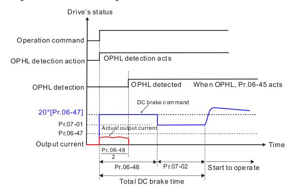
• Status 4: The drive is in STOP; Pr.06-48 ≠ 0; Pr.07-02 = 0 When the drive starts, it executes Pr.06-48 as the DC brake. The DC brake current level is 20 times the Pr.06-47 setting value.
