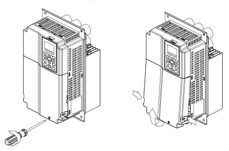
Frame C Screw torque: 12–15 kg-cm / (10.4–13 lb-in.) / (1.18–1.47 Nm)
