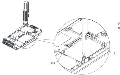
Remove the two screws as shown in the figure on the left.
