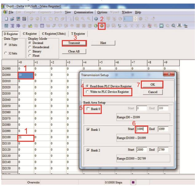
Another method can be used to set D1091: Determine which of slave stations 0 to 7 will not be needed, and set the corresponding bits to 0. For instance, if it is not necessary to control slave stations 2, 6 and 7, merely set D1091 = 003B, and the setting method is the same as described above: Use WPL to initiate
