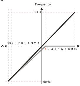
Pr.00-21=0 (Digital keypad control and run in FWD direction) Pr.03-05 Analog Positive Voltage Input Bias (AUI) = 10% Pr.03-07~03-09 (Positive/Negative Bias Mode)
