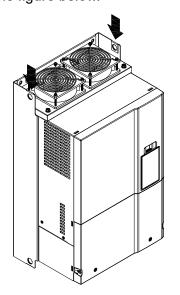
Pay attention to the installation method of lifting hook, avoid the lifting holes of the drive deforming due to improper installation. See the figure below.
