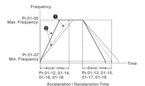
① Optimize the acceleration / deceleration time when Pr.01-44 is set to 0.
