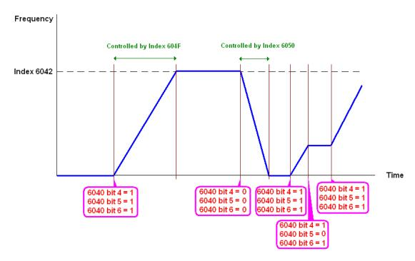
NOTE 01: To know the current rotation speed, read 6043. (unit: rpm)
