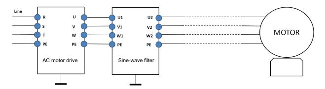
Figure 7-14 Wiring of non-shielded cable
