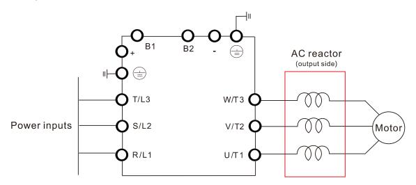
Figure 7-13 Wiring of AC output reactor
