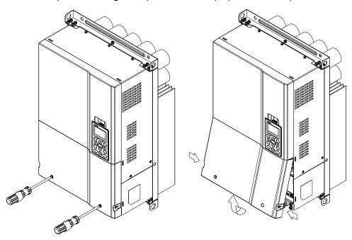
**Step 2**Frame A–D Screw torque: 6–8 kg-cm / (5.2–6.9 lb-in.) / (0.59–0.78 Nm)
