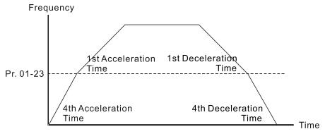
1st/4th Acceleration/Deceleration Frequency Switching
