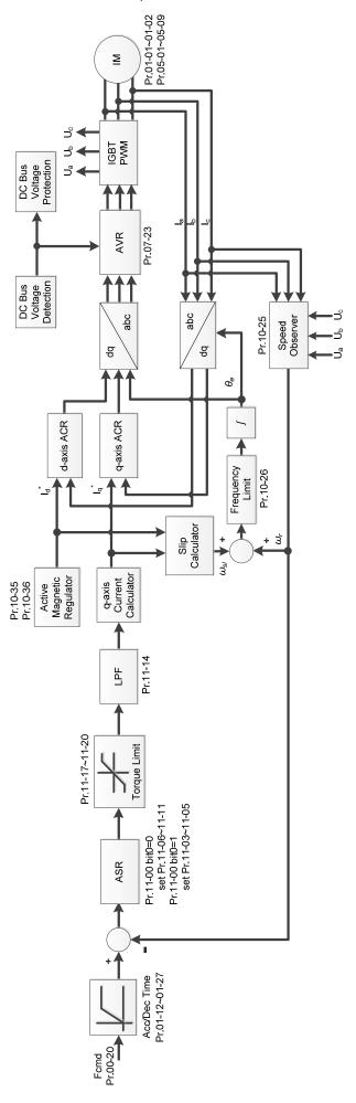
When Pr.00-10 = 0, and you set Pr.00-11 to 6, PM FOC Sensorless control diagram is as follows:
