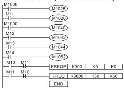
■ Parameter 09-33 are defined on the basis of whether reference commands have been cleared before PLC operation
