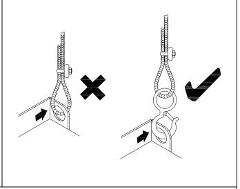
Pay attention to the angle between the lifting hole and the lifting hook, see the figure below. Applicable to VFD450CT43A00C; VFD550CT43A00C
