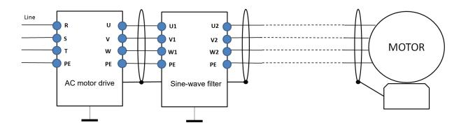
Figure 7-15 Wiring of shielded cable
