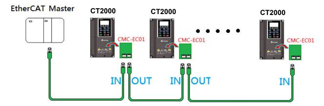
When the hardware is installed and power on, check for the display. The current set value of Pr.09-60 will be 6, and shows "EtherCAT" on the display. If the above information does not show on the display, check the version of CT2000 (V3.05 and later) and the connection of the card.
