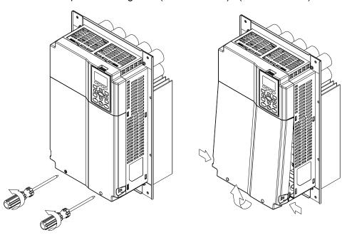
Frame D Screw torque: 10–12 kg-cm / (8.7–10.4 lb-in.) / (1.0–1.18 Nm)
