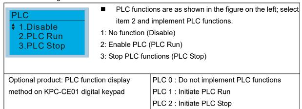
■ When the external multifunctional input terminals (MI1 to MI8) are in PLC Mode select bit0 (51) or PLC Mode select bit1 (52), and the terminal contact is closed or open, it will compulsorily switch to the PLC mode, and keypad switching will be ineffective. Corresponding actions are as follows:
