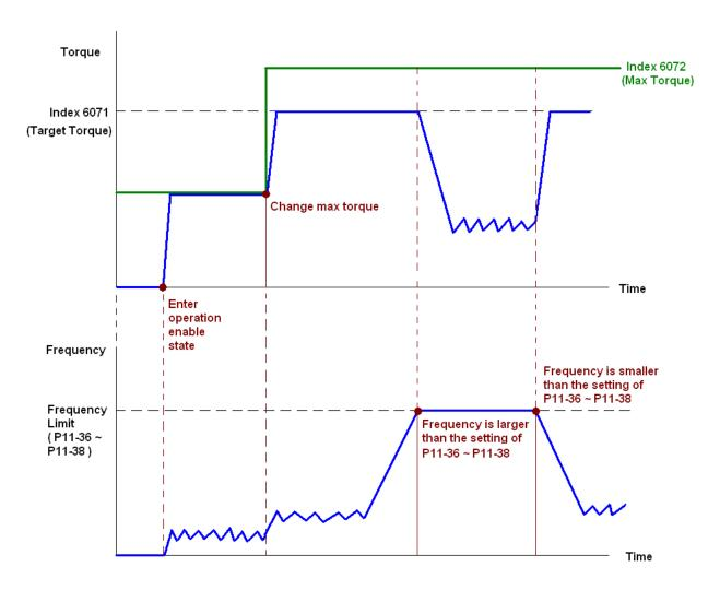
NOTE: The standard DS402 doesn't regulate the highest speed limit. Therefore if the motor drive defines the control mode of DS402, the highest speed will go with the setting of Pr11-36 to Pr11-38.
