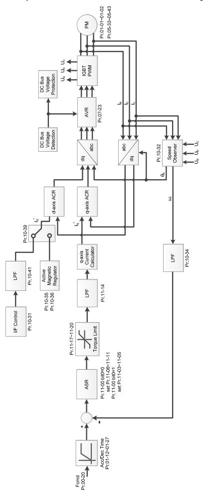
When Pr.00-10 = 0, and you set Pr.00-11 to 7, IPM FOC sensorless control diagram is as follows:
